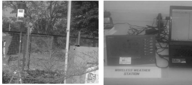
(a) Developed system and Referenced Weather station outdoor unit. (b) Developed system and Referenced Weather station indoor unit.
